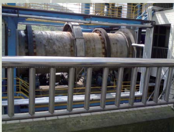
回转窑高温焚烧技术 Rotary kiln high temperature incineration technology 等离子体反应器 Plasma reactor
