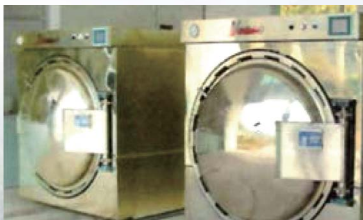
医疗废物高温高压灭菌锅 High temperature and high-pressure medical wastes sterilizers
