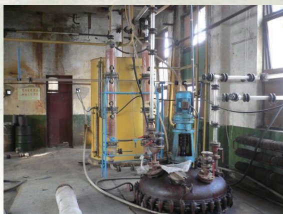
非封闭系统三氯杀螨醇生产设备 Non-closed facility for dicofol production
