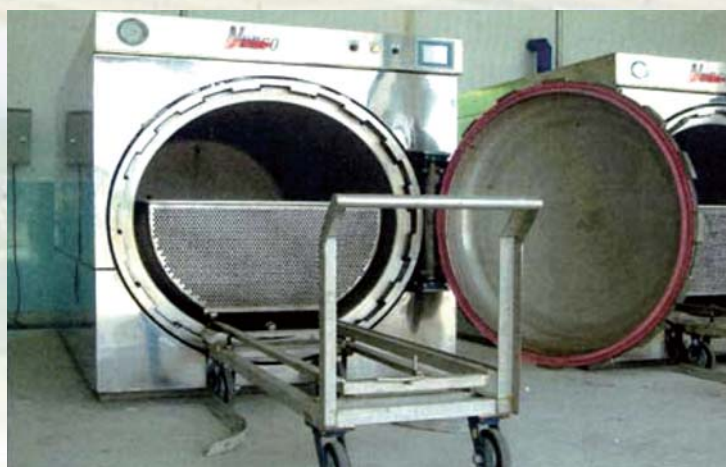
医疗废物高温高压灭菌锅 High temperature and high-pressure medical wastes sterilizers
